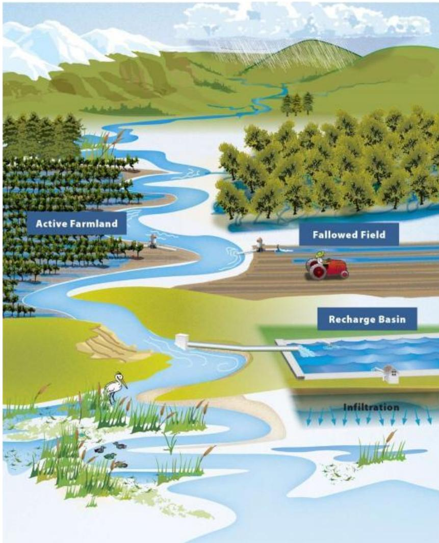
[This schematic illustrates different ways managed aquifer recharge can be accomplished. \(Source: California Department of Water Resources\)](#) One way to do that is by [managed aquifer recharge](#), or MAR. Surface water or flows from storm-swollen rivers are steered onto land where the water percolates into the ground. It is a straightforward process that works within the right parameters, experts say.
